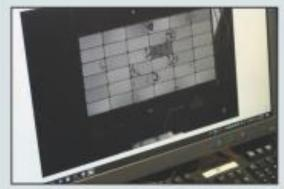
A brand-new 36-cell panel is subjected to electroluminescence testing. The camera reveals an underperforming cell and some microscopic cracking.
