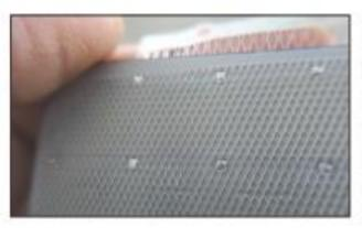
A Merlin MTAT energycollection grid for the back side of a solar cell—with many connection points and short energy paths to the grid—lowers resistance, increases efficiency, and can significantly minimize the effects of any cell cracking and other damage.
