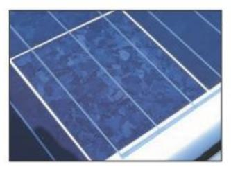
The bluish color and multiple alignments of the crystals in this rigid panel clearly indicate that these are polycrystalline, or multicrystalline, cells.
