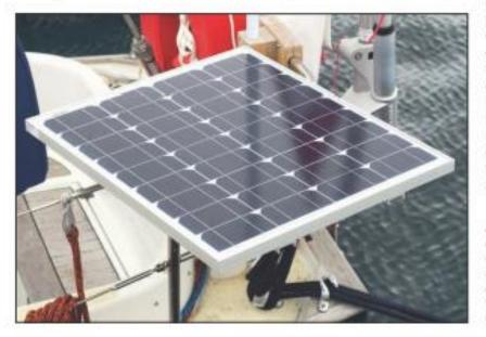
An adjustable stern rail mount holds a conventional rigid solar panel (fingers and busbars on the top of the panel). Again, these are half cells to boost the voltage to battery-changing levels in a relatively small panel.
