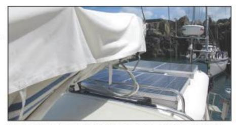
The author's four nominally 12V panels are wired in series and parallel for 24V. The output of the two panels overshadowed by the boom is knocked down by 50%, and the total array by 25%.
