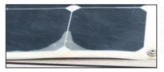
Delamination of a semi-flexible solar panel is a common failure. Once again, these are SunPower Maxeon cells.
