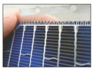
The MTAT copper grid structure, best thought of as a network of springs connected to the front and back of the cell, with a series of compliant springs linking adjacent cells to each other, adds a considerable measure of stability to the otherwise brittle silicon cell wafers. It minimizes the failures associated with traditional soldered conductors. In the event of
