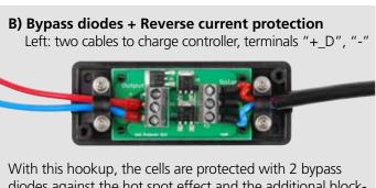
With this hookup, the cells are protected with 2 bypass diodes against the hot spot effect and the additional blocking diode protects against reverse current back into the module. By damage to a module or cable by several modules in parallel operation, an influence can be prevented on the other modules with the use of the blocking diode.
